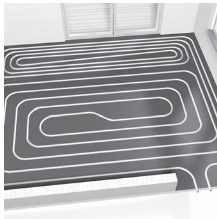
Figure 3: Snail's shell installation pattern with integrated peripheral area
